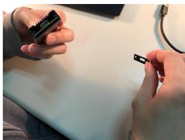
2. At 30-degree angle, Insert the M.2 SSD magnetic pin into the M.2 Port of the unit
