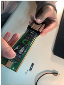
5. Place the cover Plate over USB port. Secure the cover plate by inserting two Screws and use screwdriver to fixed the screws.
