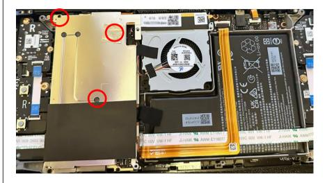
5. Prior to proceeding, disconnect the Steam Deck battery to ensure safety.
