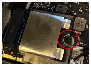
7. Transfer the ESD Shielding from the old SSD to the new SSD and Install the new SSD securely.
