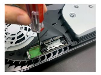
7. Attach the expansion slot cover and fasten the screw (A).
