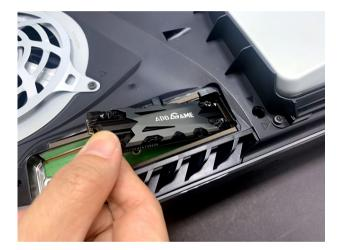
Please Make sure the SSD is firmly inserted all the way into the expansion connector. If not, it may cause damage to your PS5 console.
